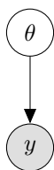
Figure 2.1: Graphical model notation for the coin example. Nodes represent random variables (white: latent, shaded: observed), and an arrow denotes conditional dependence between them. In this case, the number of heads depends probabilistically on the weighting of the coin.
