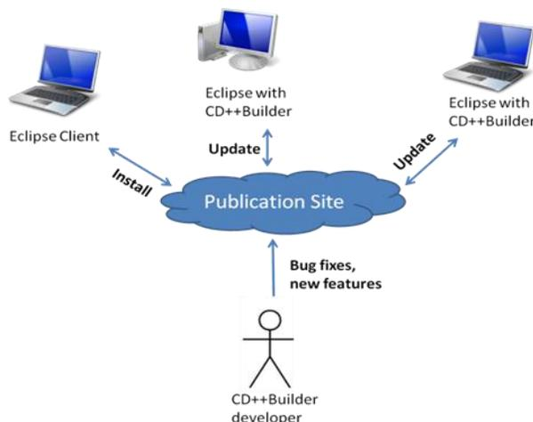
Figure 7. Centralized installation and update architecture.
